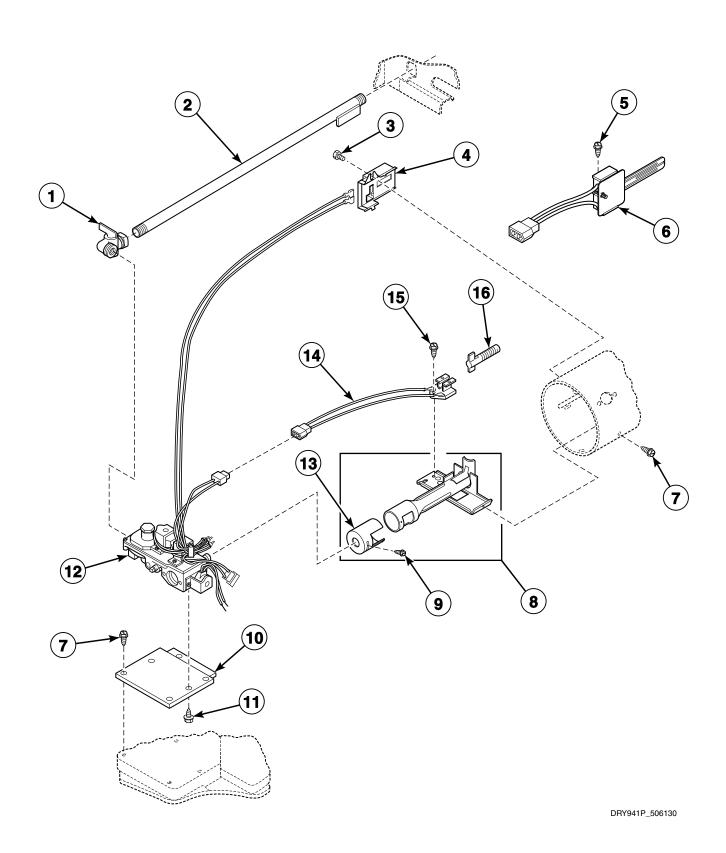
**56279 Gas Valve Assembly**Models RG5190, RG5192, RG5290, RG5292, RG6190, RG6192, RG6192-3000, RG6292, RG6390, RG6392 and SG5190
