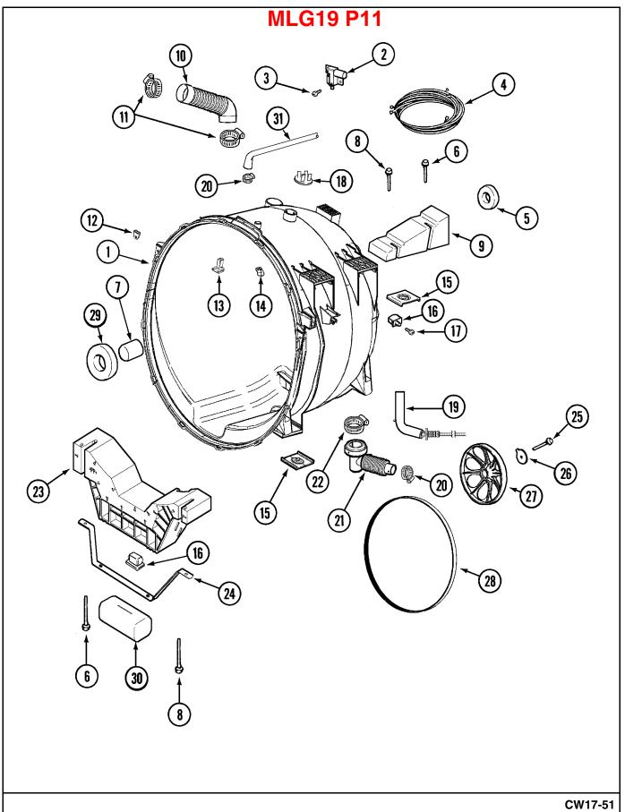
Section: SPINNER ASSEMBLY & OUTER TUB COVER(WASH)
