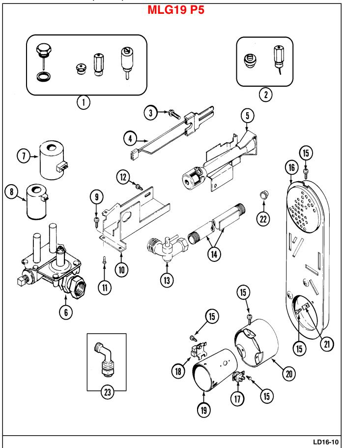
Section: MOTOR DRIVE (DRYER)
