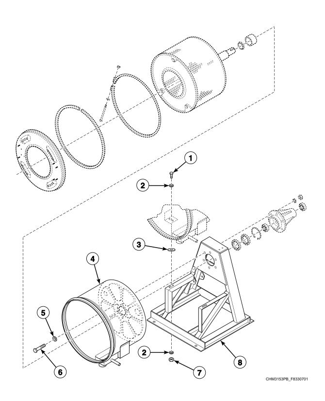
Basket, Shell, Frame and Bearing Housing - Design 2 and 3 Models (Drawing 1 of 3)
