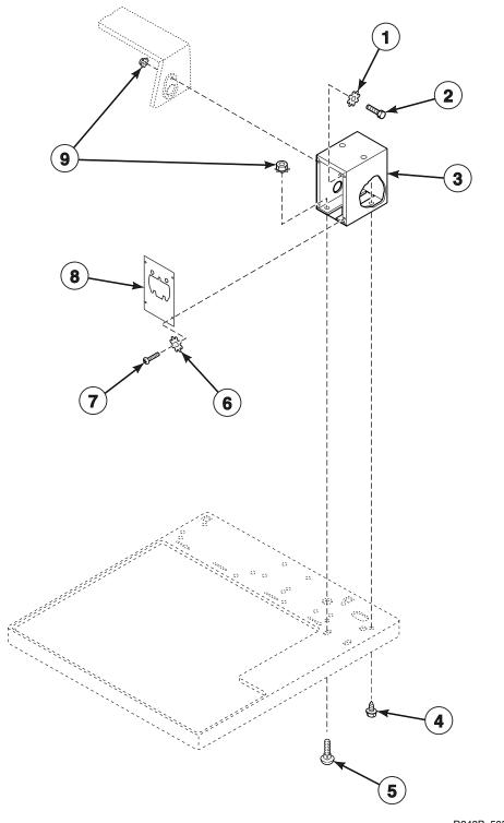
**Security Case and Card Reader**Models HDE707\*A1502, HDE707\*A1702, HDE707\*C1502, HDE707\*C1702, HDG709\*A1102 and HDG709\*C1102
